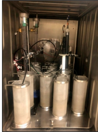
Figure 3. Cylinders used in the experiment (see Figure 2)—each one housing a specific sensor—placed inside the climatic chamber. Note: image prior to the placement of the control cylinder (explanation in the text).
