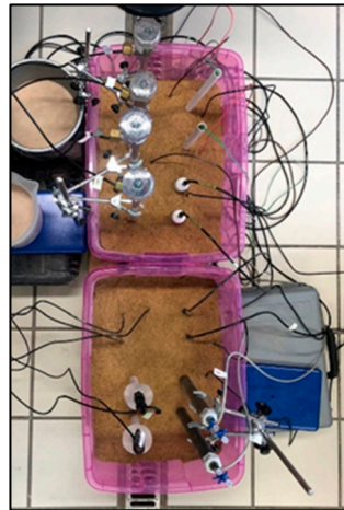
Figure 4. Experimental setup for the repeatability and reproducibility study (Test 2). In two plastic containers ( 60 \times 40 \times 30 cm) with sand, the different pairs of homologous sensors were inserted together with humidity probes (see more details in the text).
