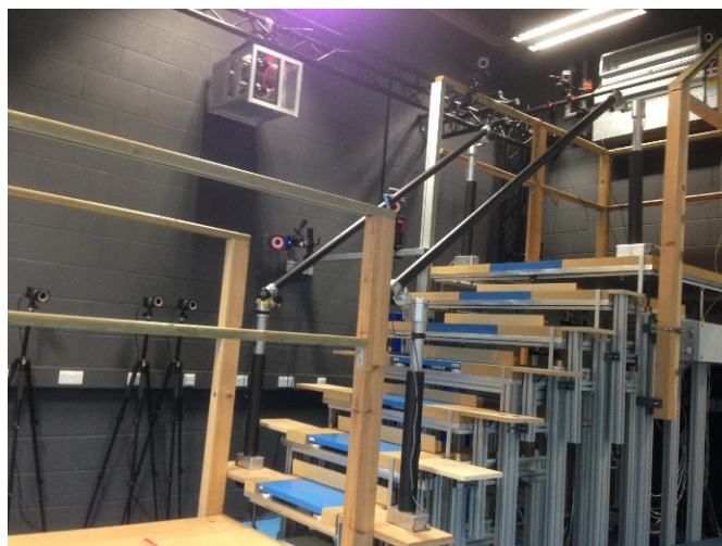
Figure 9. Laboratory custom-built instrumented seven-step staircase, first four steps fitted with a force plate, and twenty-four infrared cameras were used around the staircase for motion capture.
