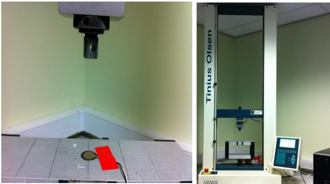
Figure S1. FSR Calibration with Tinius Olsen material testing machine.
