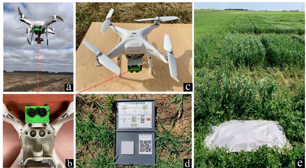
Figure 2. UAV systems and their setup in the field. (a) DJI Phantom 4 pro and attached Sentera double 4K sensor; (b) Sentera double 4K sensor (zoomed view); (c) DJI Phantom 4 pro (top view); (d) Micasense calibrated panel; (e) white poly tarps as ground control points (GCPs).
