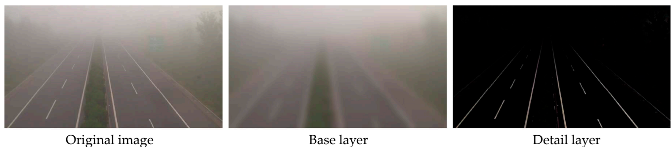
Figure 2. The original image, base layer, and detail layer. The detail layer is the detailed structural feature which we want.
