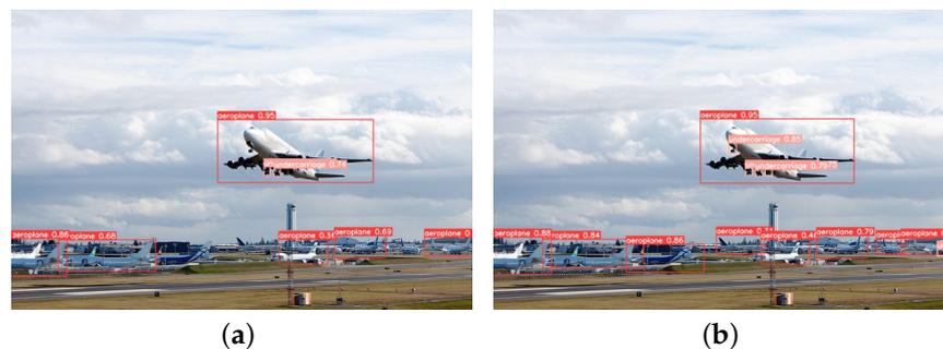
**Figure 9.** Long-range targets detection. (a) YOLOv5 detection results; (b) YOLOv5-RSC detection results.
