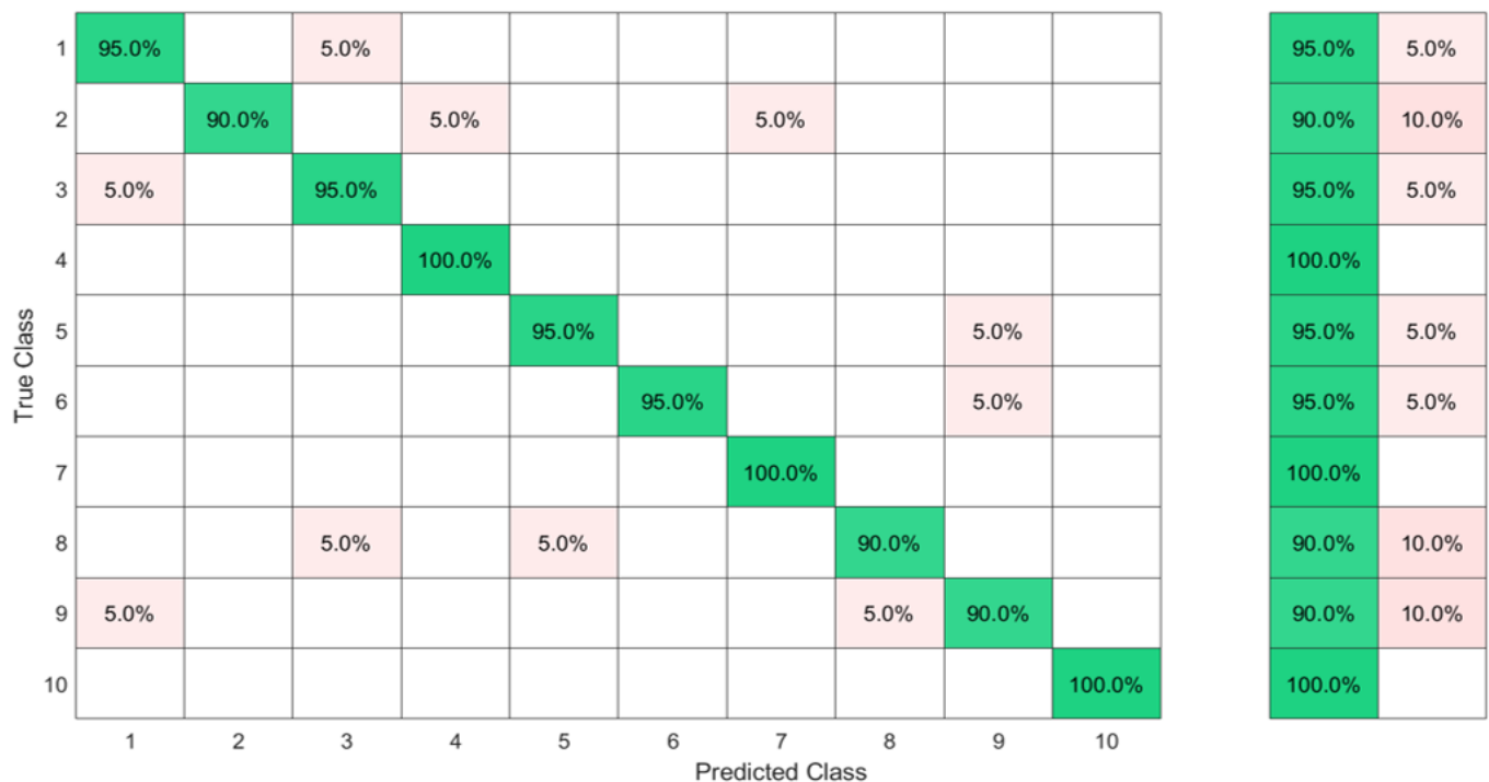
Figure 9. Ten ASL letters, A–J, detected with FMG and classified by the ELM after feature selection by the KTGELM.
