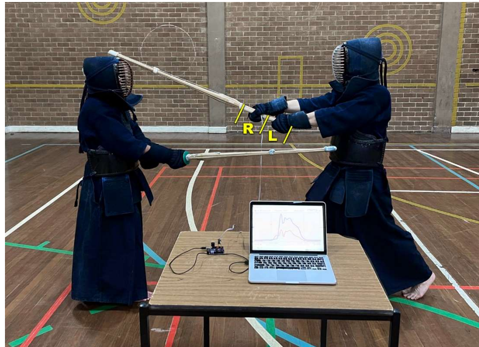
Figure 2. Experimental setup for testing the grip force with Smart Shinai (Men-bu, head target); L = pressure sensor of left hand, R = pressure sensor of right hand.
