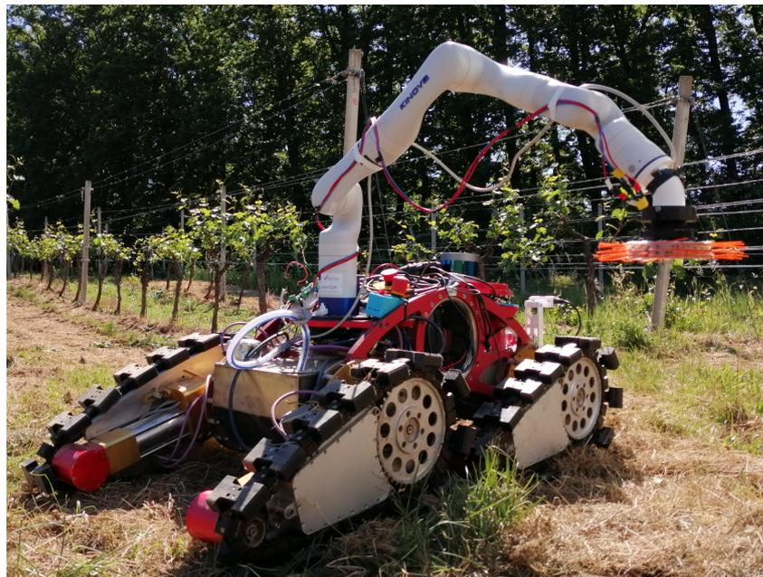
**Figure 2.** Mobile manipulator developed as a part of the HEKTOR project. Direct drive brush-shaped tool is mounted as a robotic manipulator end-effector.
