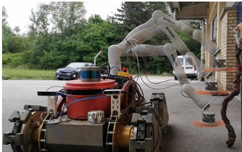
**Figure 8.** Trunk following experiment. Compliant control in forward direction from Section 4 is used, while the tool follows a sinusoidal function in the vertical direction.
