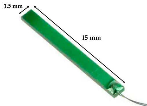
Figure 9. Bimorph piezoelectric beam used in the experimental setup: RS 285-784, RS Component. Dimensions: length 15 mm, width 1.5 mm, and thickness 0.6 mm.
