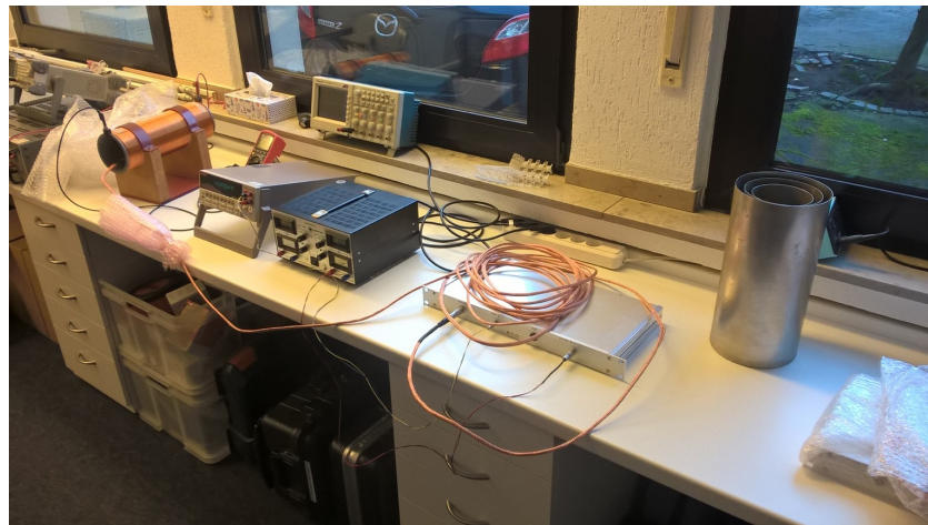
Figure 9. Acceptance test setup, the solenoid is visible on the left, the zero-gauss chamber is visible on the right.
