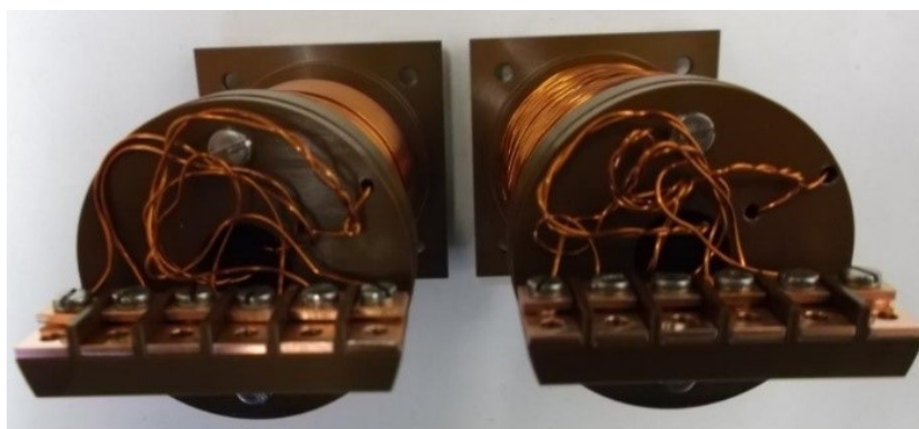
Figure 7. Picture of the coil windings around the peek reel, showing the system for the connection to the external cable.
