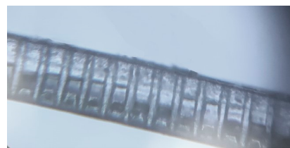
Figure 6. Microscope image of the LPG on the small core (250 \mu\text{m} ) POF following a non-use period of three months.
