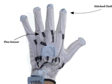
Figure 2. Placement of flex sensors in glove for hand gesture data.
