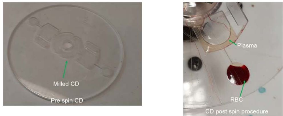
Figure 5. (Left) The image of the fabricated CD before the blood sample is loaded. (Right) The image of the part of the disc with RBC chamber and the reciprocation chamber after blood plasma separation has been performed—the red blood cells are all separated in the RBC chamber as is evidenced by the dark red color, while plasma only (transparent fluid) is present in the reciprocation chamber. The nitrocellulose membrane that is normally present in the reciprocation chamber has been removed to improve the clarity of the image.
