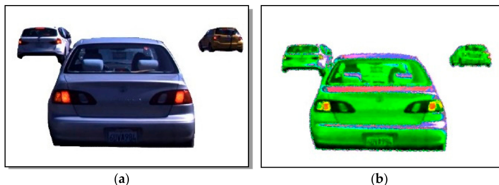
Figure 6. Example results of energy features: (a) background-subtracted image and (b) energy features.
