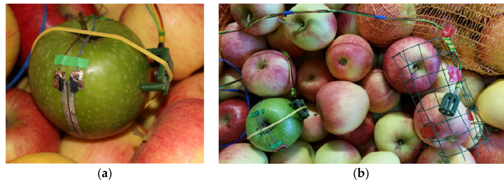
Figure 2. Wetness sensor and infrared sensor at the measuring apple (a) and grouping of the sensors in the upper layer of the apple bin (bottom left, wetness sensor and infrared temperature sensor attached to the same apple; bottom right, air temperature and relative humidity sensor) (b).
