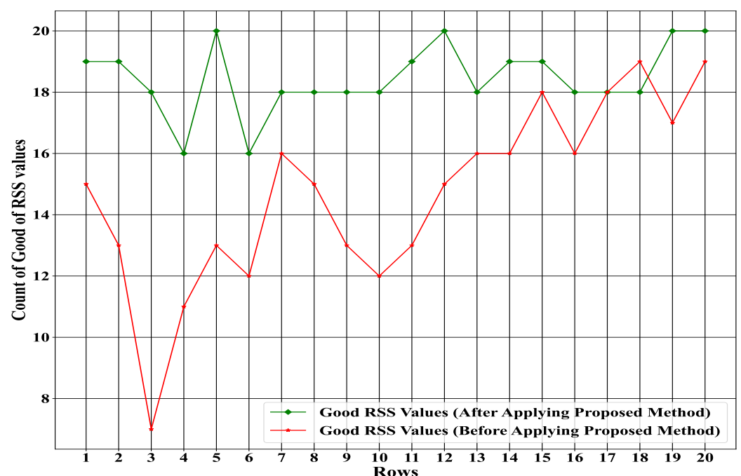
Figure 10. Improving the number of good RSS values before and after applying the proposed method.
