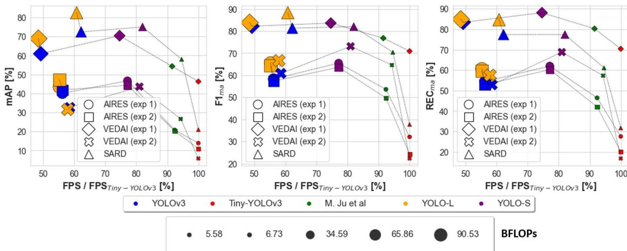
**Figure 9.** Performance summary of the different networks on AIREs, VEDAI and SARD datasets as a function of FPS. The marker size is proportional to the BFLOPs required by the network. For a better readability, FPS is normalized by Tiny-YOLOv3’s speed [3]. The model denoted as M. Ju et al. can be found in [3].
