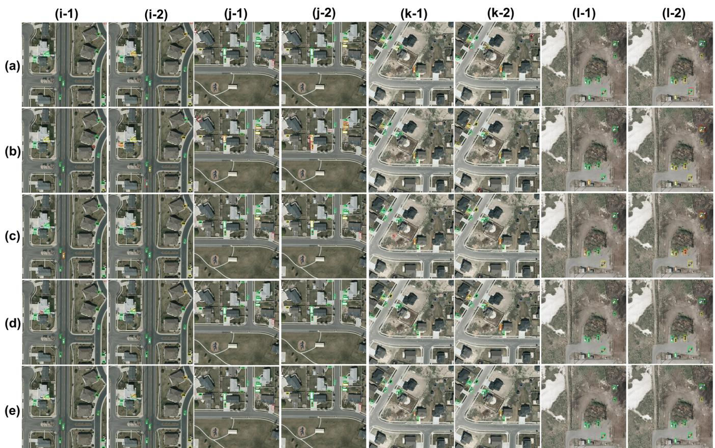
**Figure 7.** Experiments 1 (odd columns) and 2 (even columns) on VEDAI dataset. Comparison of different CNNs: (a) YOLOv3; (b) Tiny-YOLOv3; (c) CNN by [3]; (d) YOLO-L; (e) YOLO-S.
