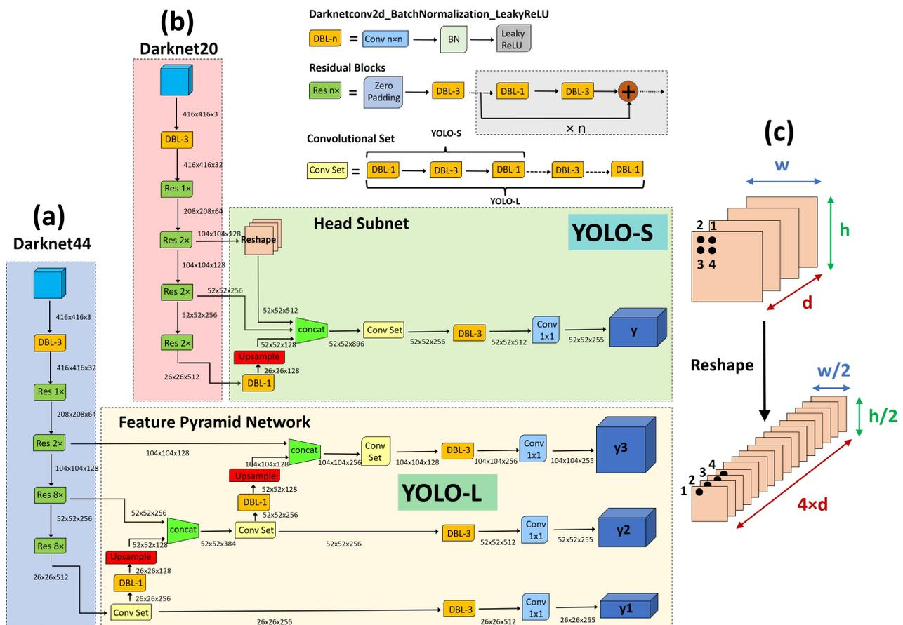
**Figure 4.** Overview of the proposed networks: (a) YOLO-L; (b) YOLO-S; (c) Reshape-Passthrough layer. In the figure,  $C = 80$  classes have been assumed (dataset COCO [37]).
