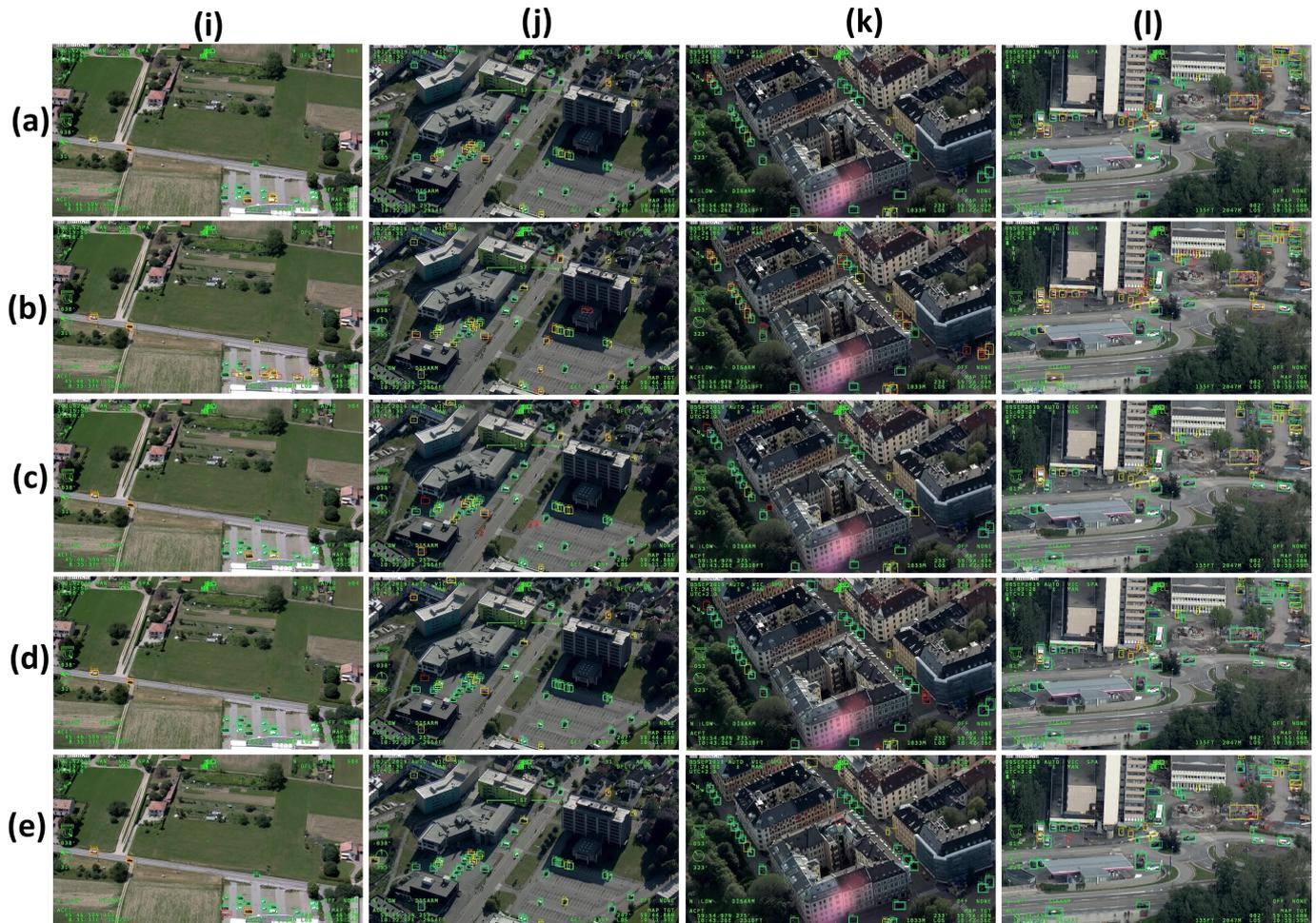
**Figure 6.** Experiment 1 on AIRES. (a) YOLOv3; (b) Tiny-YOLOv3; (c) [3], (d) YOLO-L; (e) YOLO-S. The following backgrounds are considered: (i) rural (Italy); (j–l) urban (Norway). Green (red) box denotes the true (false) positives, whereas the ground truth box is depicted as a light blue box if detection is correct and as a yellow box if a false negative occurs.
