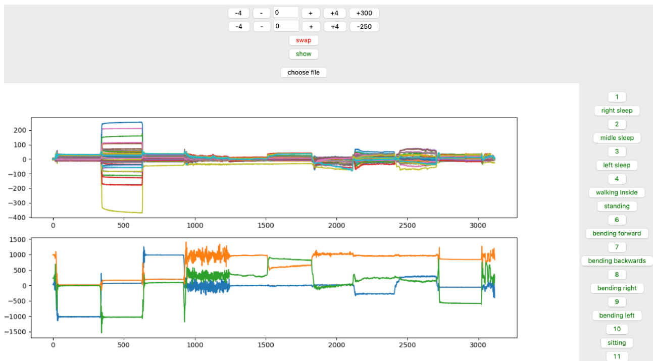
Figure 5. GUI for labeling indoor data. Time stamps and all three categories of activities are interactively configured and selected on the top and right side of the GUI, respectively; and in order to label the data, buttons on the right side of the panel can be used.
