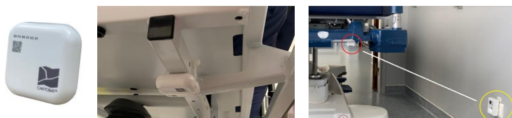
Figure 5. A typical tag mounted on a stretcher. The yellow circle in the right figure shows a plugged CartoModule.
