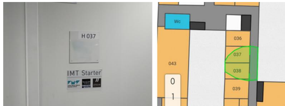
Figure 4. The principle of coupling mapping and location: the green surface is the resulting location which does not require any calibration or model design. On the left is the “visual” location of the tag, and on the right is the area calculated by the system (in green).
