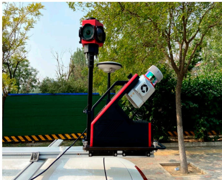
Figure 6. The vehicle-mounted laser measurement system SZT-R1000.
