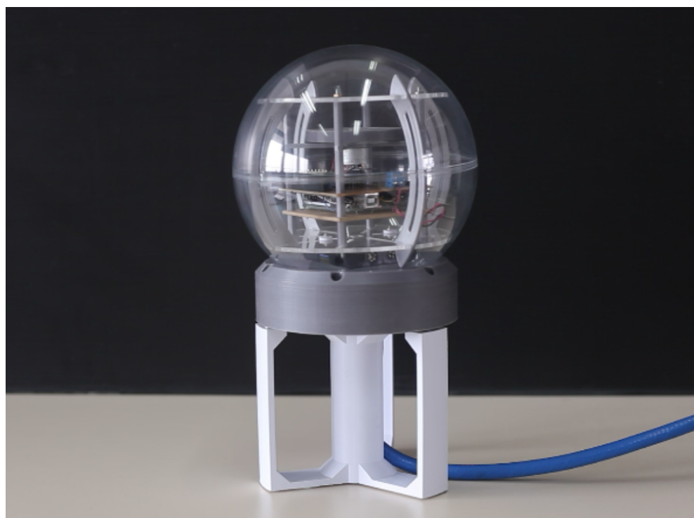
Figure 8. Photograph of the ADCS model used for experimental verification of the presented attitude estimation algorithm based on gradient descent and complementary filter.
