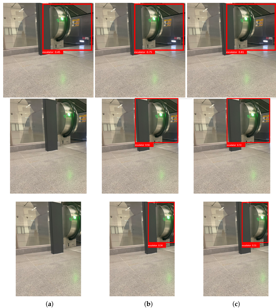
Figure 4. Comparison analysis results of the context-aware object detection algorithm and conventional object detection scheme for the escalator and glass door: (a) Yolo V4; (b) Faster RCNN ResNet 50; (c) Proposed system. From top to bottom, the occlusion conditions are shown from low, medium, and high levels.
