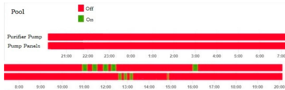
Figure 8. Pump panels pump and purifier pump start-up time for scenario 3.
