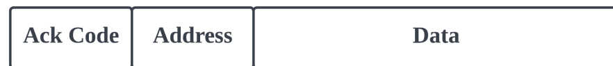
Figure 5. Message payload components. The message payload consists of three components: the acknowledgment (Ack) code, sender address, and data.
