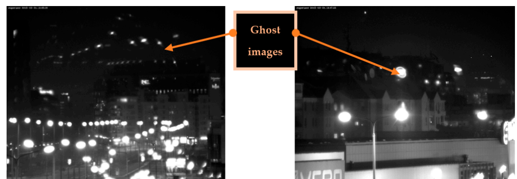
Figure 10. Optical protective window without AR coating (ghost images are visible).
