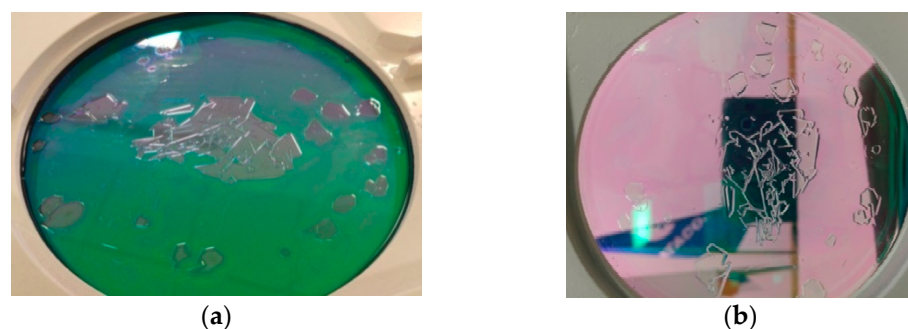
Figure 11. Optical protective window AR coating damage: (a) in transmitted light; (b) in reflected light.
