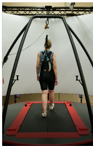
Figure 1. An example of the experimental setup with one individual using the CAREN system. The platform can be translated in the mediolateral direction during a participant walking on the treadmill in the anteroposterior direction.
