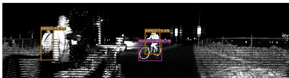
(b) YOLOx detection results on a sample image from the reflectivity channel.
