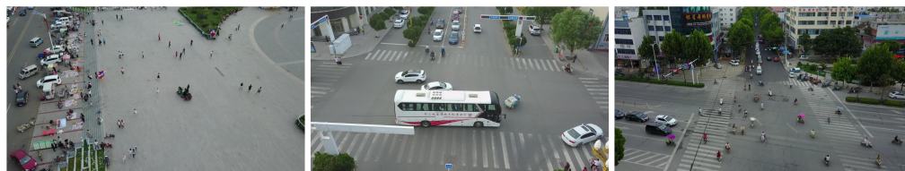
Figure 1. Object detection issues in UAV aerial images: a high proportion of small objects, multi-scale objects, a high overlap between objects, and complex backgrounds.
