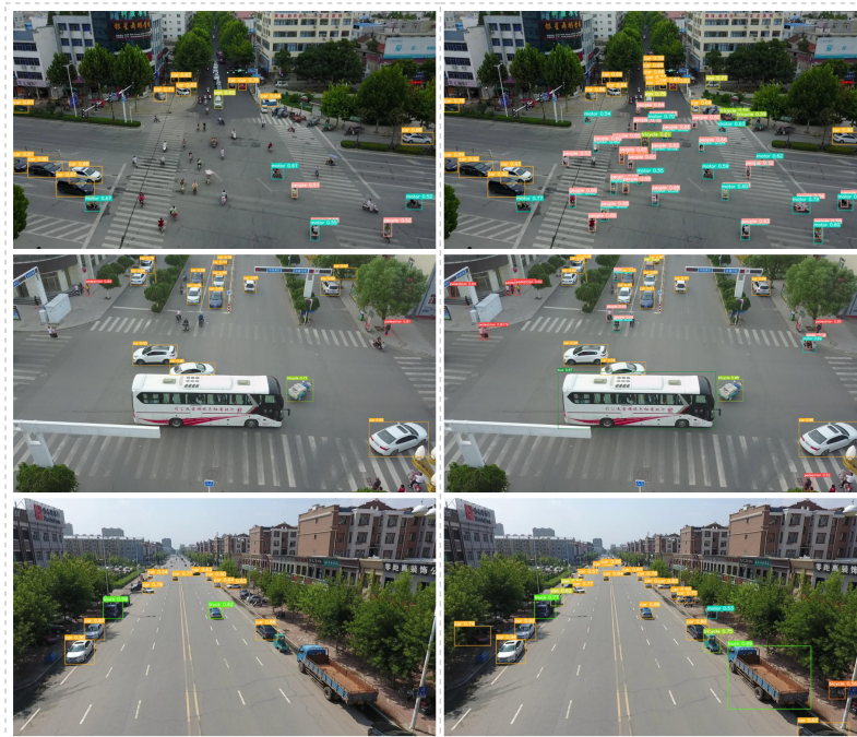
Figure 9. Picture detection effect comparison chart (the picture on the left is the result of direct detection by YOLOv5s and the picture on the right is the result of our improved model detection).
