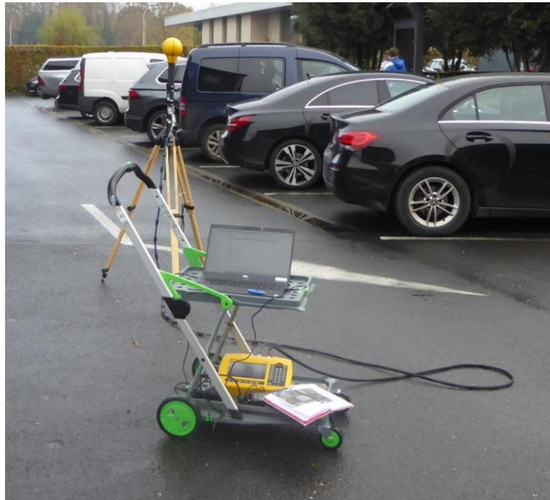
**Figure 2.** Second type of equipment used in this study to measure the exposure to 5G new radio base stations, consisting of a Narda SRM-3006 field strength analyzer (SRM) and a tri-axial isotropic antenna (“probe”).
