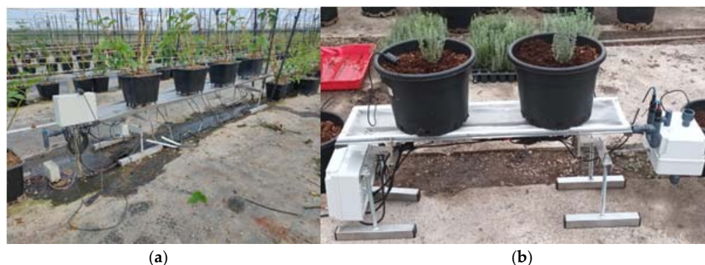
Figure 13. (a) Weighing tray with torsion load cells in a Mexican commercial fruit facility. (b) Small weighing tray in a commercial facility in the South of Spain.
