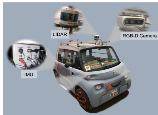
Figure 3. The Citroën AMI modified by the ESIG-ELEC for data recordings.
