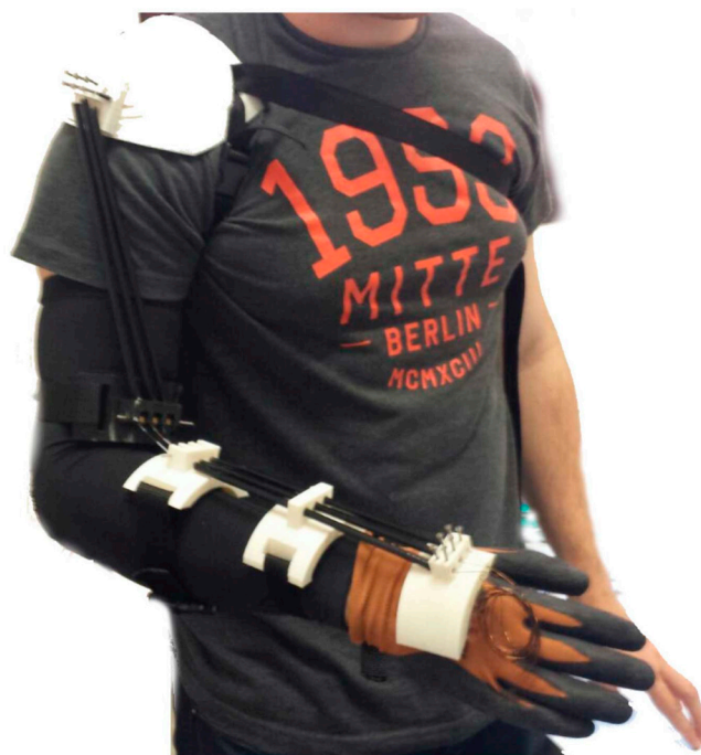
Figure 6. Illustration of a SMA-driven soft wearable. Copaci et al. [142] describe their work on a SMA-driven rehabilitative elbow wearable. SMA wires serve the same function as cables, providing a contractile force for joint motion. In their work, the process of heating the SMA wire takes 4.5 s while the cooling phase takes 25 s.
