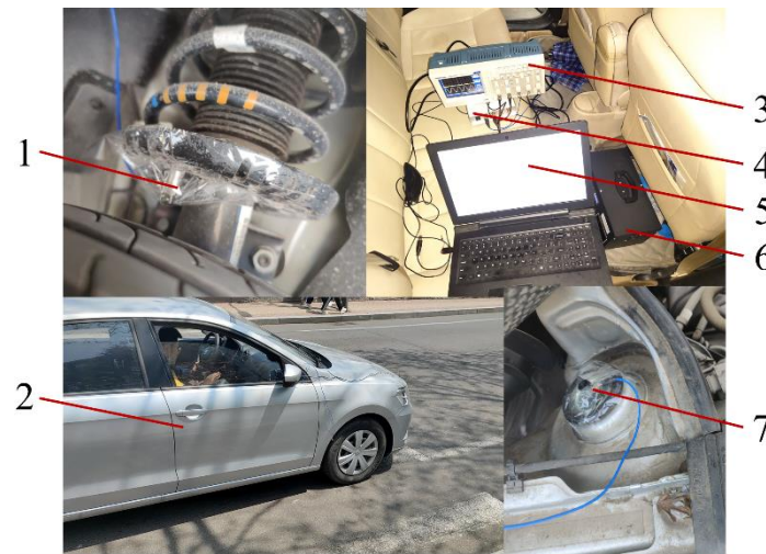
Figure 9. Test vehicle and test equipment diagram. 1/7. Acceleration sensor 2. Test car 3. Digital oscilloscope 4. Data acquisition card 5. Upper computer 6. External power supply.
