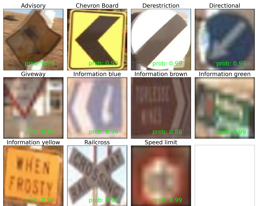
Figure 6. Examples of TP detected and TP classified traffic signs for each class. Softmax Estimated Probability (prob) is provided for each in green. Although extracted traffic signs vary in size and resolution, our pipeline still manages to classify correctly with above 95% test performance and strong estimated probabilities in a multinomial setting.
