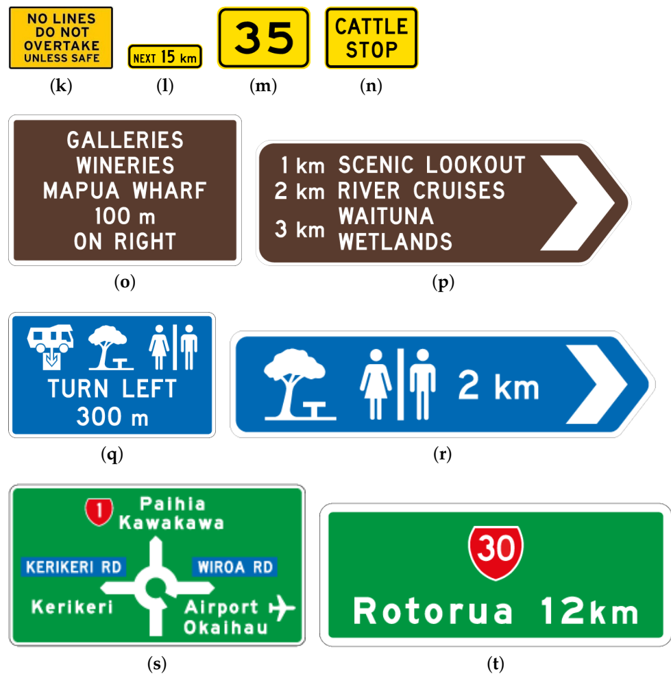
Figure 5. Examples of the traffic signs [60] (a,b) being classified as Chevron boards, (c–e) as Advisory, (f) as Give way, (g) as Railcross, (h) as Directional, (i) as Speed limit, (j) as Unrestricted, (k–n) as Information yellow, (o,p) as Information brown, (q,r) as Information blue, and (s,t) as Information green.
