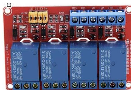
Figure 6. Photovoltaic generation system: 4-relay modules of on/off actuator.
