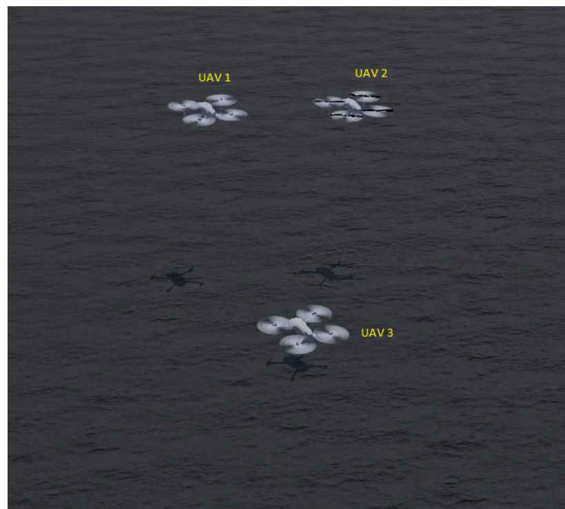
Figure 10. An illustration of multi-robot pursuit–evasion scenario where UAVs 1 and 2 have captured and “grounded” UAV 3, which is an evader robot.
