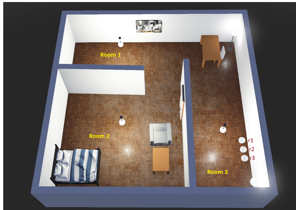
Figure 12. An illustration of multi-robot task allocation: there are 3 iRobot Roombas ( r1 – r3 ) and 3 rooms to clean. In a one-to-one matching scenario, the objective would be to assign one Roomba to a certain room. However, as room 2 is larger in size, two robots might be needed to clean it, whereas the third robot ( r3 ) might be assigned to rooms 1 and 3.
