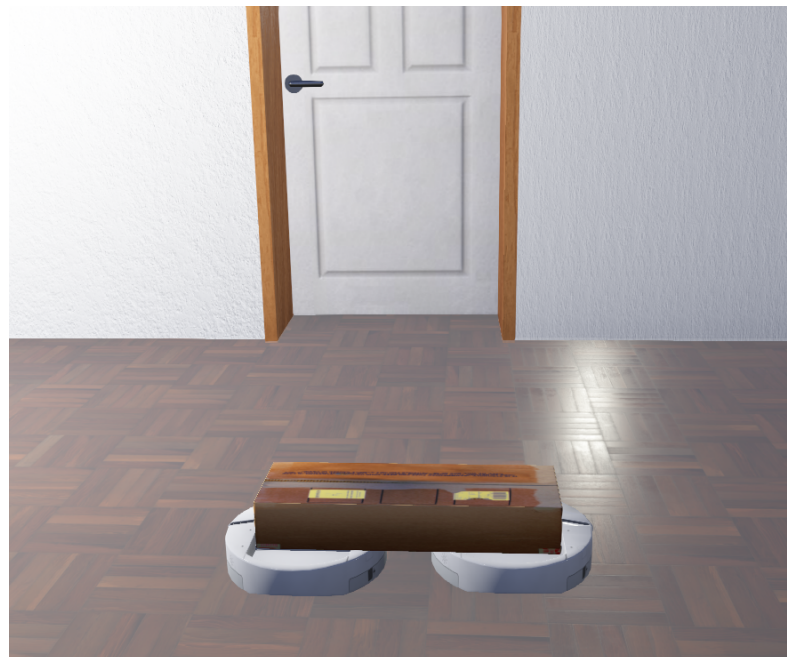
Figure 13. An illustration of multi-robot object transportation is presented where 2 iRobot Create robots carry a cardboard box and plan to go through a door in front of them.
