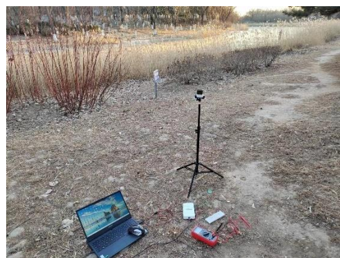
Figure 11. Experimental setup for scattered solar radiation experiment.
