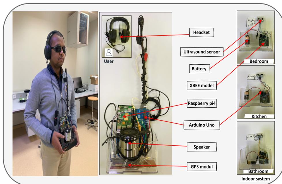
**Figure 2.** Prototype of the wearable smart system.
