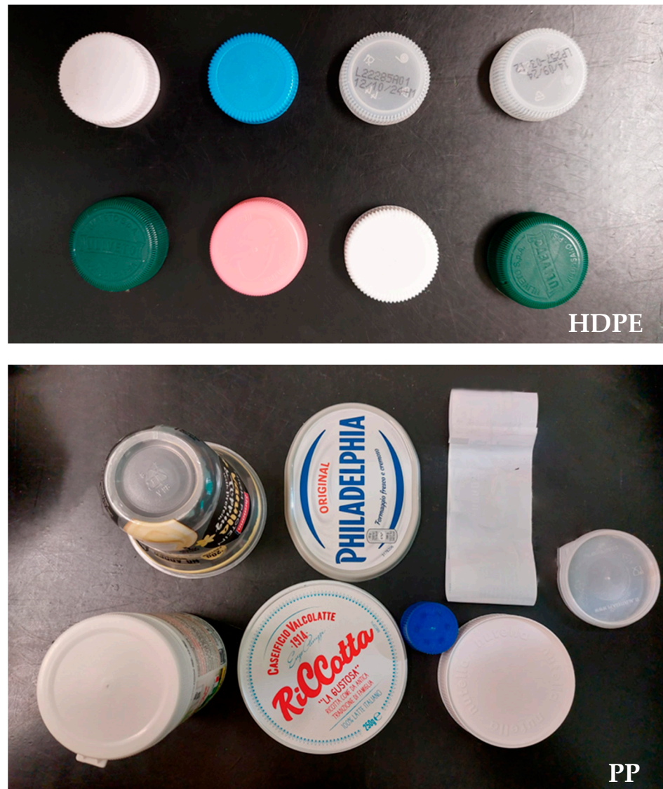
Figure 8. The plastic samples used for the test of the microplastic sensor.
