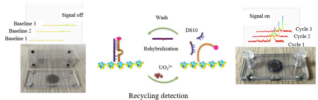
Figure 3. Ultra-sensitive recyclable SERS microfluidic biosensor for the detection of \text{UO}_2^{2+} [62].
