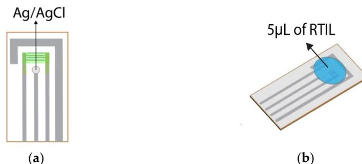
**Figure 7.** The preparation before measurement: (a) Applying Ag/AgCl ink as RE; (b) Dropping 5  $\mu$ L of RTIL as electrolyte.
