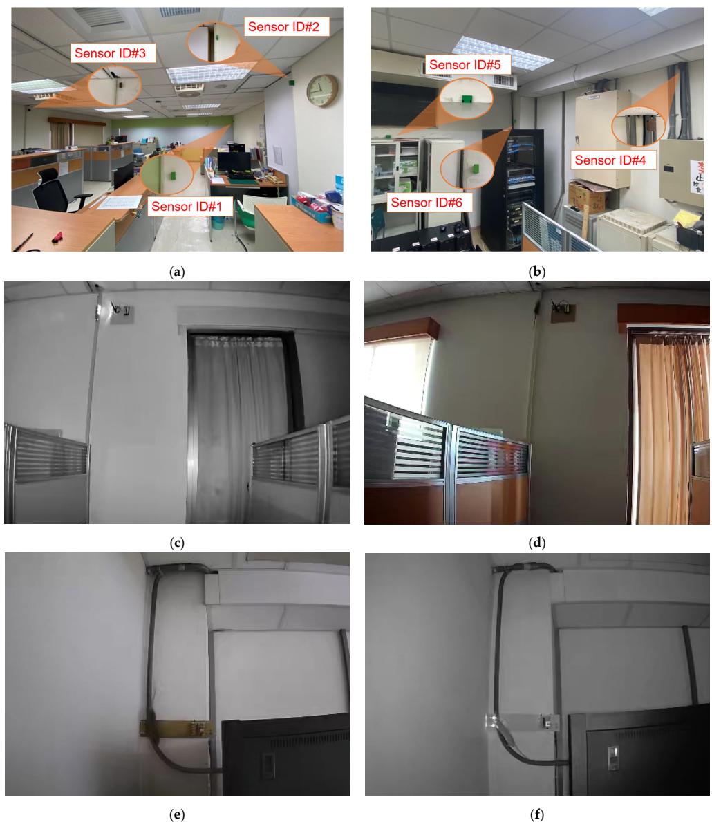
Figure 16. Setup and detection photos of rodents' activity in different buildings: (a) sensor setup position in building 1; (b) sensor setup position in building 2; (c) mouse forward action detected in building 1; (d) mouse backward action detected in building 1; (e) mouse forward action detected in building 2; (f) mouse backward action detected in building 2.
