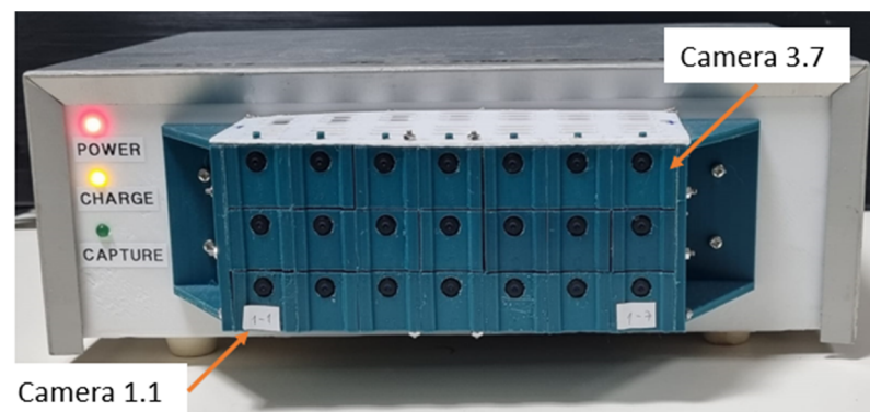
Figure 4. The array imaging system with 7 \times 3 mini cameras used for computational integral imaging [31].
