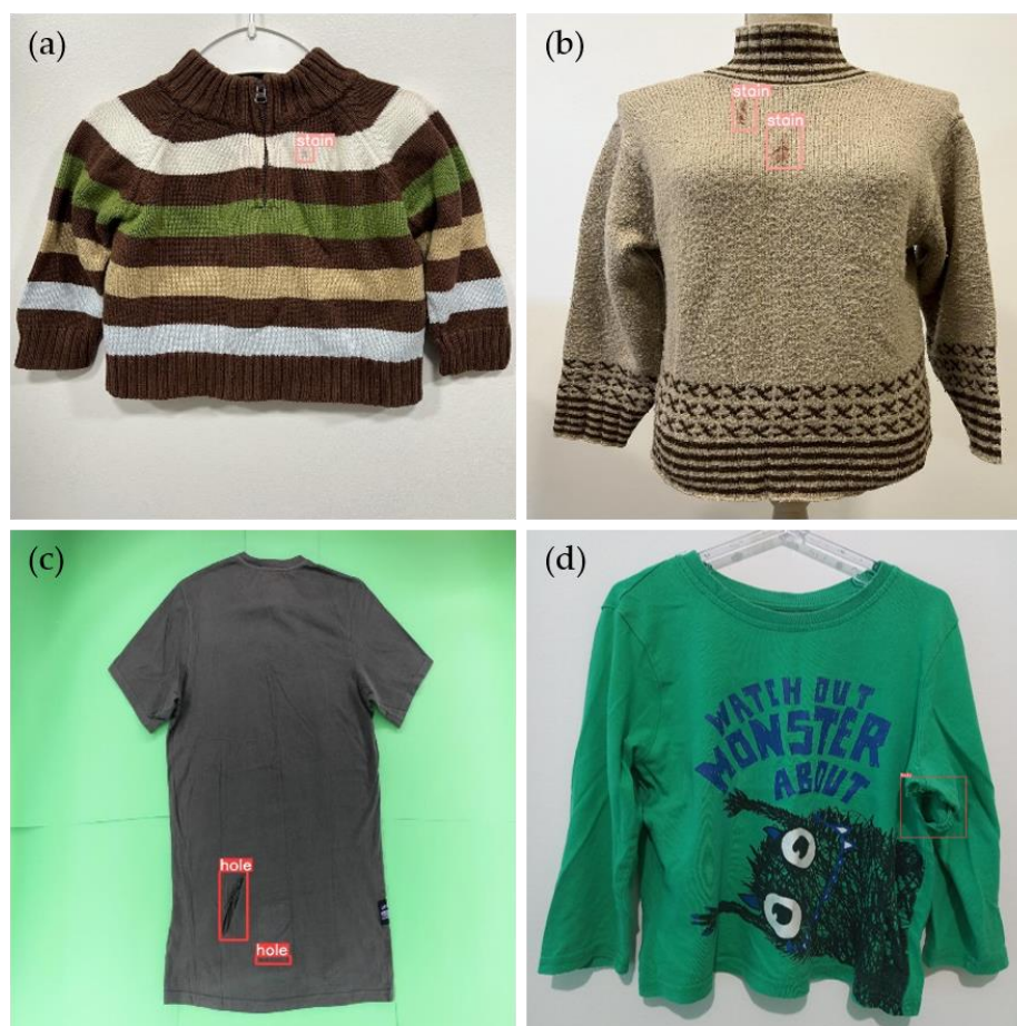
Figure 8. Examples of predicted images from the YOLOv5l6: (a) single stain detection, (b) multiple stain detection, (c) multiple hole detection, and (d) hole detection near the seam.
