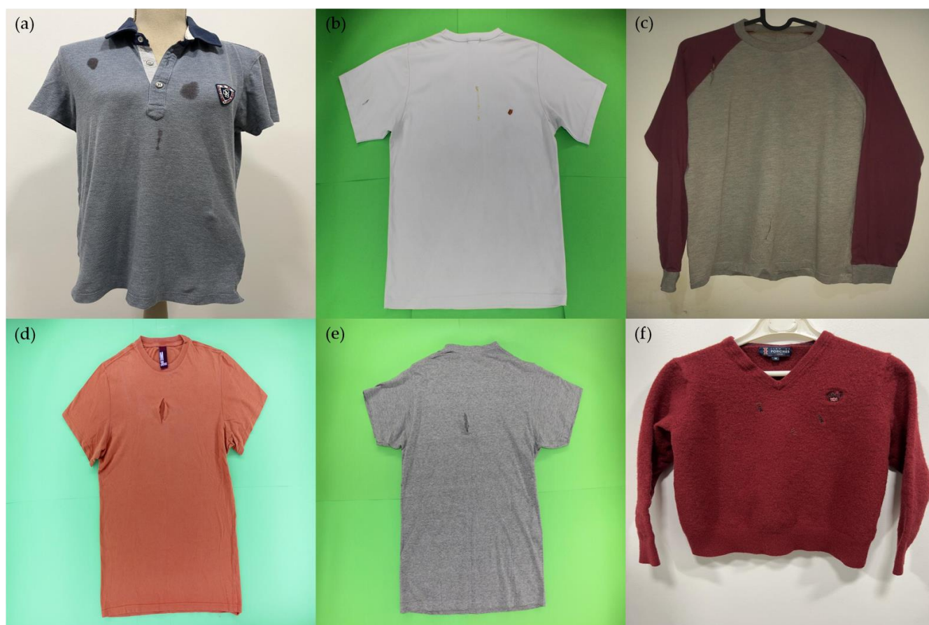
Figure 4. Examples of sample images from the dataset, demonstrating different types of defects and distributions, with variations in backgrounds and illumination conditions: (a) multiple stain defects, (b) a combination of stain and hole defects, (c) multiple hole defects, (d) a single hole defect, (e) hole defect on the backside, and (f) multiple hole defects.
