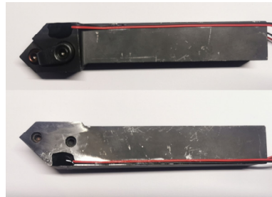
Figure 3. Cutting tool holder with affixed semiconductor strain gauge.
