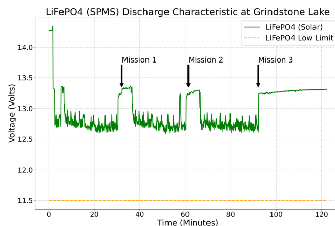
Figure 11. Solar battery system performance at Grindstone Lake on 18 May 2022.
