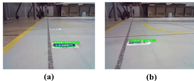
Figure 11. Detection of turning induction markers. (a) Case 1 of turning induction marker detection; (b) Case 2 of turning induction marker detection.
