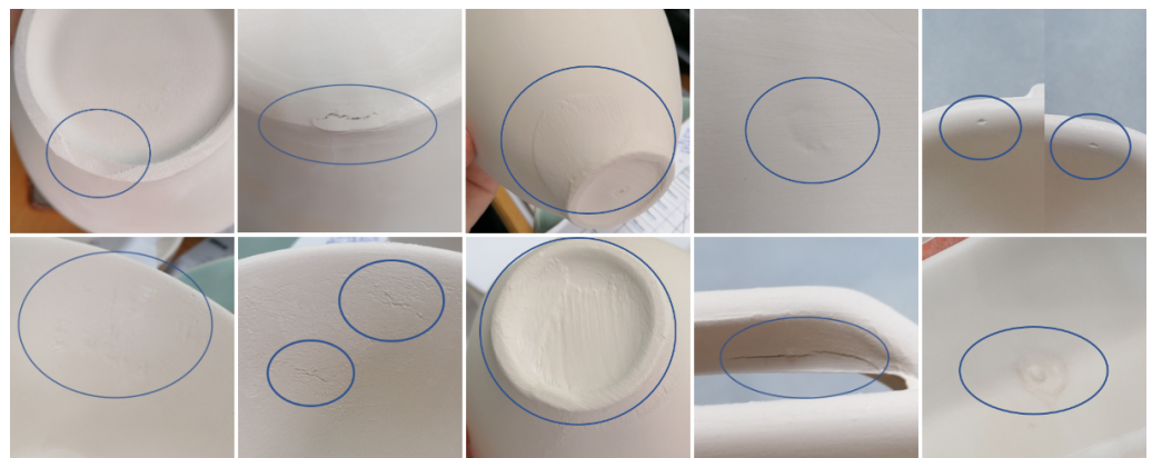
Figure 3. Examples of different defect categories that arise during the manufacturing process.
