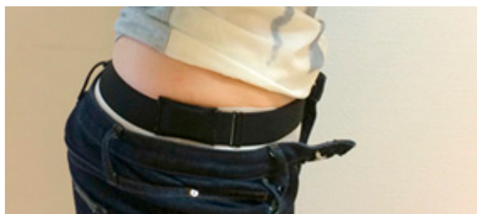
Figure 1. The placement of the accelerometer at the level of the iliac crest on an elastic hip-band.
